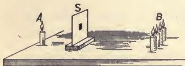
FIG. 202. — Showing a Method of Measuring the Candle Power of Lights.
